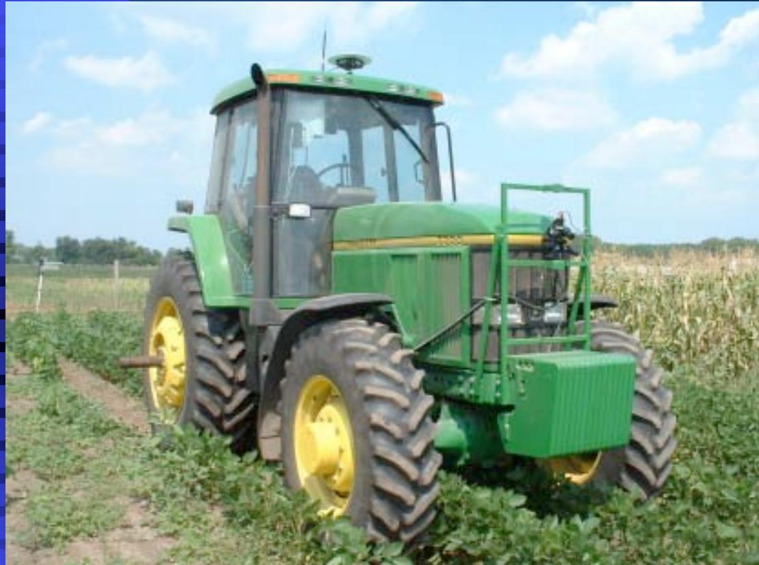
Stereo camera mounted tractor<sup>1)</sup>
