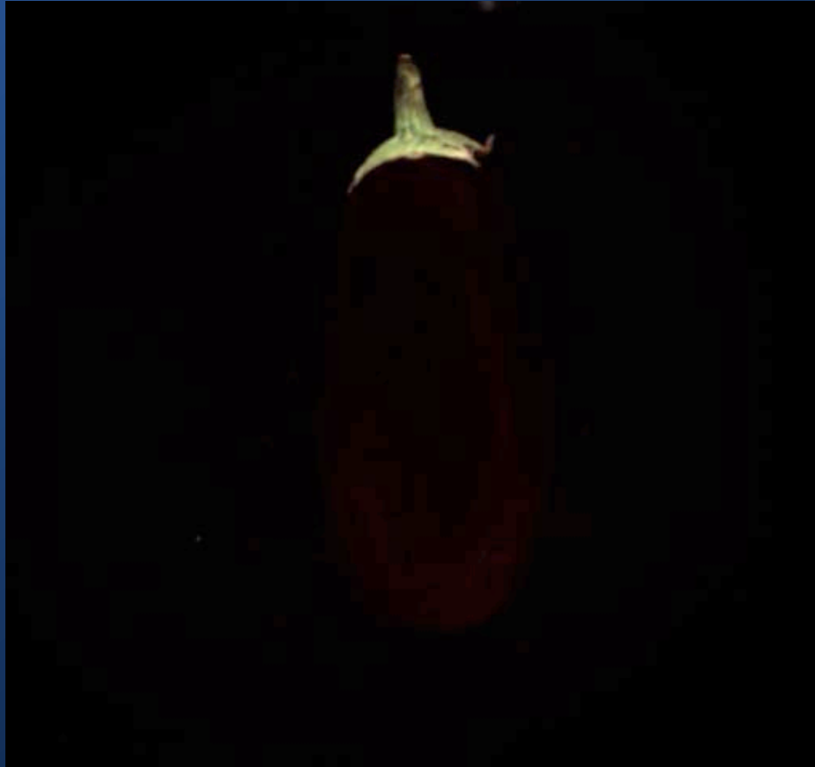
PL filtering image (Two PL filters are used in front of camera and light)
