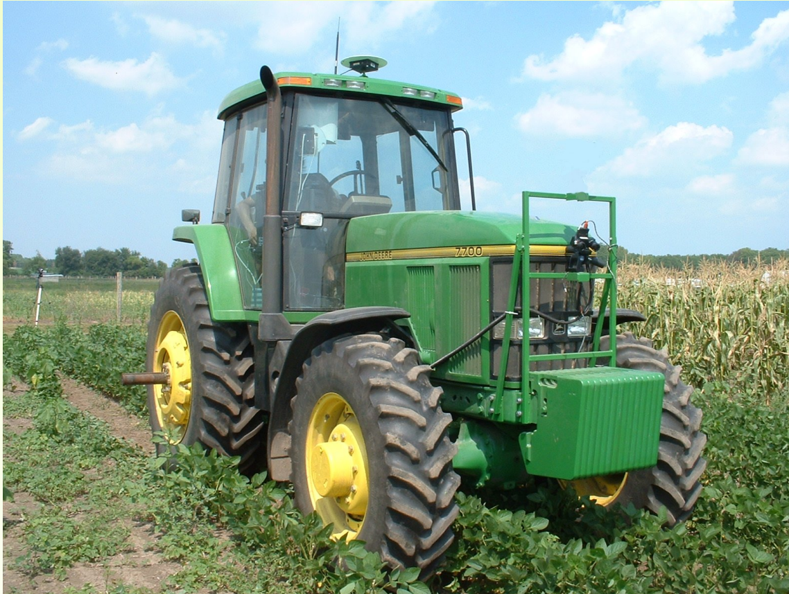
Stereo camera mounted tractor 1)
